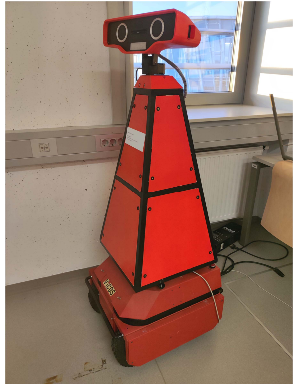
Fig. 7. ATRVmini robot used in the experiments. A model of the robot was used in the simulation, and the policy was tested on the real robot. The robot is equipped with a laser range scanner and localization beacons, among other equipment.
