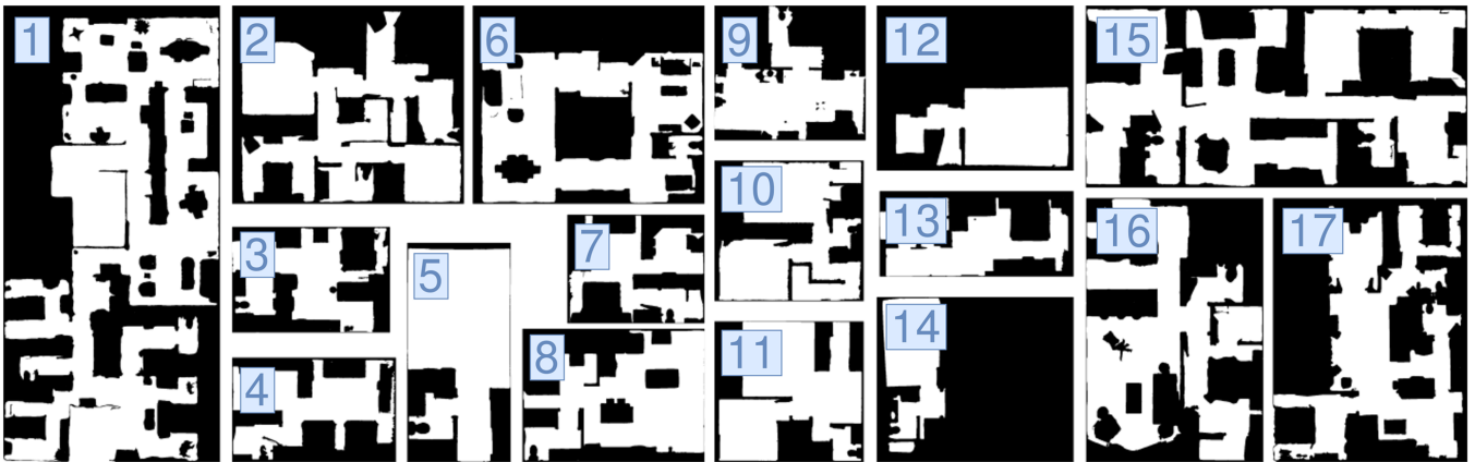
Fig. 9. Visualizations of all 17 environments in the IN2D dataset used for the evaluation of the navigation methods. The environments are real floor plans of 3-D scanned indoor spaces and contain realistic configurations of various obstacles. These maps were loaded in the ROS, and a simulation of the ATRVmini robot was navigated on each map.
