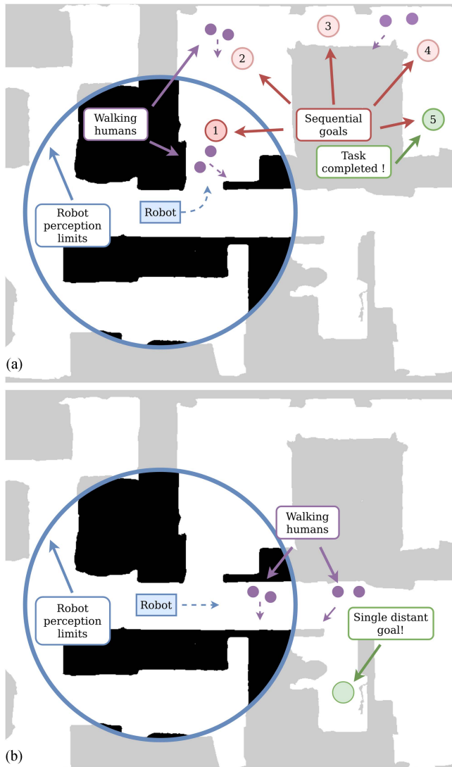
Fig. 8. (a) Long episode experiments. The robot knows only the next goal, and after reaching it, it is supposed to navigate to the next goal. The episode is successfully completed when the final goal is reached. (b) Second type of experiment when a single distant goal is provided to the robot. Both settings become dynamic when the visualized pedestrians are added to the simulation.
