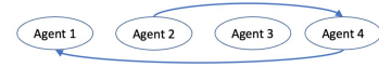
Fig. 19. Scenario for AMR-IAC where a subset of agents communicate with each other. We apply one-agent-at-a-time rollout with the agent order \{2, 4, 1\} , and we apply the base policy for agent 3.
