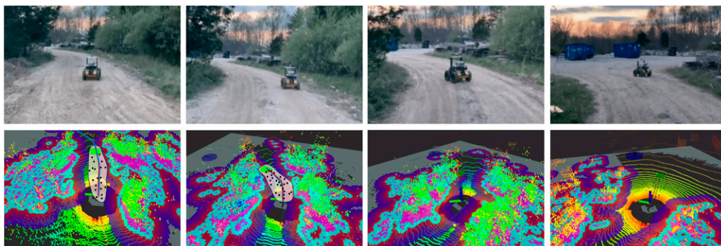
Figure 14. Snapshots of navigation in a trail using trajectory sampling to sample the states and cost map to represent the environment. The visualization in the second row shows the cost map as a 2D color map, where a darker color means a higher cost. In the first two visualizations, thickened/emphasized annotations are overlaid on top of the cost map. Specifically, the red and blue trajectories represent the expected path by executing the policy and the global path, respectively. The scattered black dots adjacent to the global trajectory represent a selected subset of sampled states, included specifically for illustrative purposes. Furthermore, the region encapsulating these states signifies the effective domain of the policy. This is defined as the area within which the value function yields a positive value. The goal for each time step is shown as a green square. The final goal is the blue circle.
